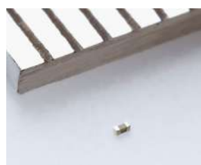
0201 size (0.25mmx0.125mm) ultra-small multilayer ceramic capacitors
